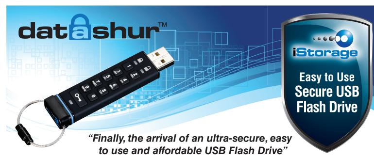
The iStorage datashur is the world's most secure, easy to use and affordable USB flash drive, employing PIN code access with military grade AES 256-bit hardware encryption. The datashur incorporates a rechargeable battery allowing the user to enter a 7-15 digit PIN onto the on-board keypad before connecting the drive to the USB port.
